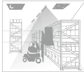
Light is on when sensor detects the motion and the ambient lux level is insufficient
