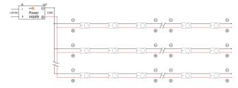
! 25 pcs - max number of modules in one chain when the power supplied from single end. ! String end voltage can't be less than 11V, do not exceed specified module string length
